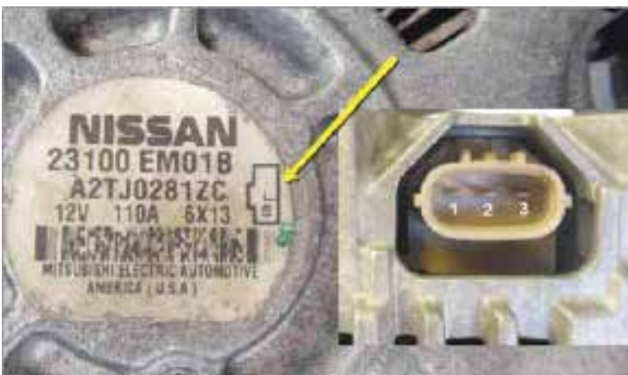
Figure 1 - Mitsubishi 11343 Alternator Tag and Regulator Pins
